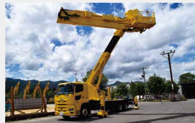
当社の橋梁点検車 Kanamoto's bridge inspection vehicle
