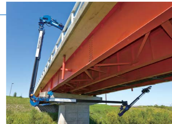
橋をはじめとするインフラの再整備は急務の課題。 写真は当社の橋梁点検車「橋竜」 Redevelopment of bridges and other infrastructure has become an urgent topic. This photograph shows Kanamoto's "Bridge Dragon" bridge inspection vehicle.
